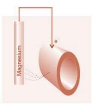
**Fig1:** Cathodic protection an anode of a more strongly reducing metal is sacrificed to maintain the integrity of the protected object (For example, a pipeline, bridge, or boat).
